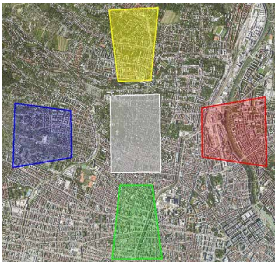
Fig. 2: Footprint of a Maltese Cross camera in the lowlands, flight direction from west to east. Nadir image = grey, oblique images = red (forward), green (right), blue (backward) and yellow (left).
