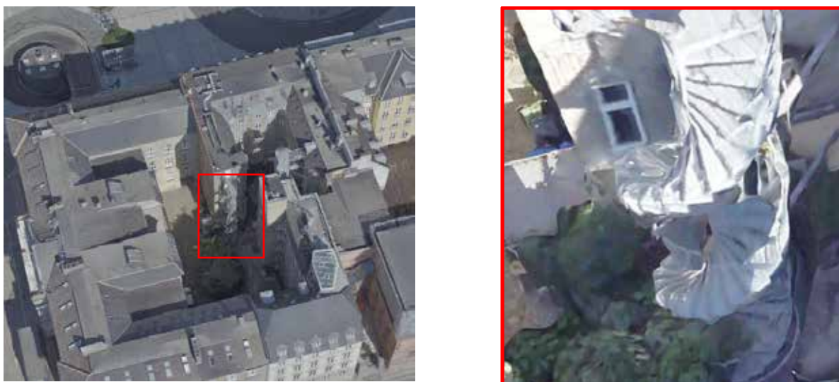
Fig. 6: Problems in the 3D mesh of Copenhagen 2021 become visible at (too) high zoom levels (right)
